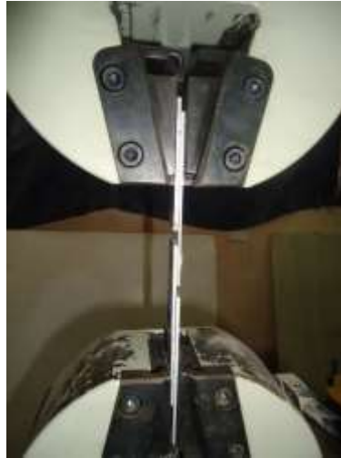
Figure 4 Tensile shear test for spot welded specimen with using shims pieces
