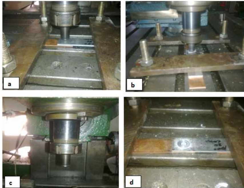
Figure 3 FSSW process steps to join the dissimilar metals of Al2024T3 and pure copper
